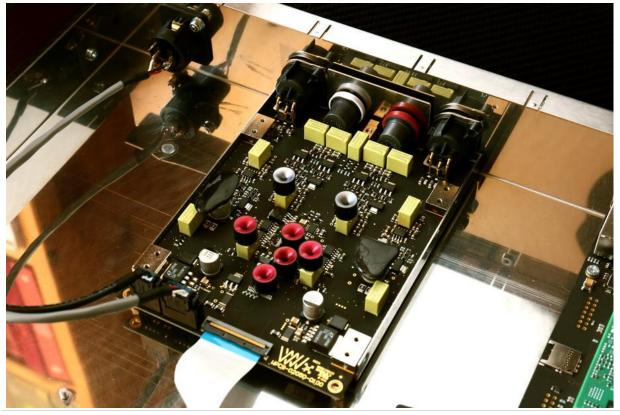
The components of the headphone output are arranged parallel to the balanced audio circuit. The signal is led from the line output and the path includes the IT OPA1611 integrated circuit and, in the output, a pair of transistors working in a push-pull system, the same as in the line output. OPA1611 works in the "unity gain" mode, ie it does not amplify the signal, but only adjusts the input impedance to the output one - it is a buffer.
