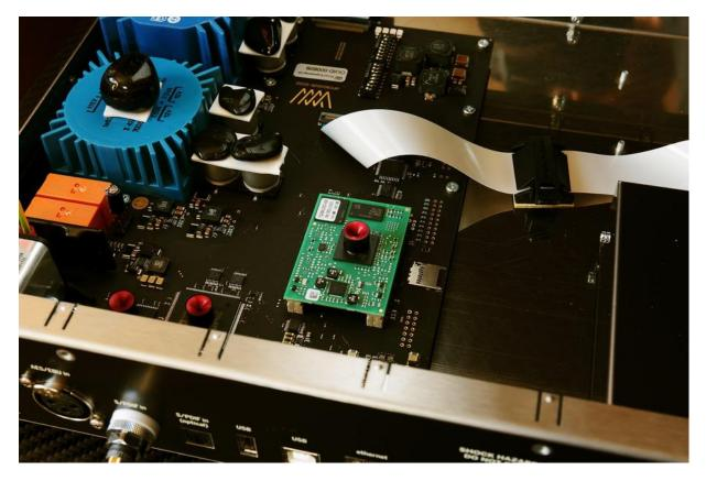
The conversion of current to voltage is performed in OT OPA1612 integrated circuits, and the output's gain and its buffering in a discrete circuit composed of medium power bipolar transistors. The system is surface mounted, while very good Panasonic relays, rarely found in consumer electronics, are threaded.
